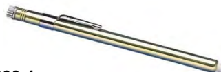
WYP800-1 Round Soapstone Holder, 1/4" X 5", Stainless Steel Inner sleeve collet securely holds the soapstone and also adjusts to grip uneven and undersized soapstone. Locking cap allows accurate adjustments for closer marking control. Sleek brass case with contrasting cap and pocket clip enhances appearance. Slim design provides better visibility in the marking area
