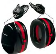
3MSH10P3E Optime™, 105 Cap-Mount Earmuffs, Hearing Conservation 10 EA/Case Pivoting ear cups for optimum fit. Twin cup design minimizes resonance, thus achieving maximum high and low frequency attenuation
