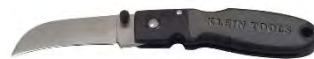
409-44004 Lightweight Lockback Knife 2-1/2" Blade is AUS8 stainless hardened to 58-59 Rc. Premium quality blade offers superior edge holding. Impact-resistant nylon resin handle with rubber insert. Reversible thumb stud provides easy one-handed opening
