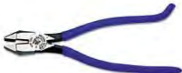
409-D201-7CST 9" Ironworker's Work Pliers Twists and cuts soft annealed rebar tie wire. Hook bend handle Spring-loaded action for self-opening Induction hardened cutting knives for long life. Hot-riveted joint ensures smooth action and handle wobble.
